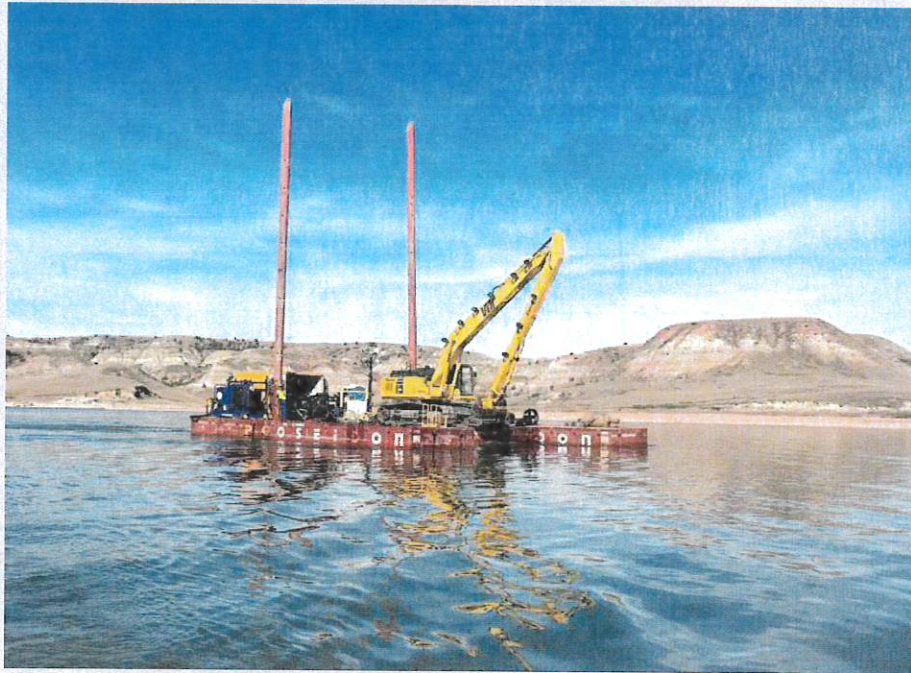
Figure 1 depicts a fully assembled flexifloat pontoon system.
