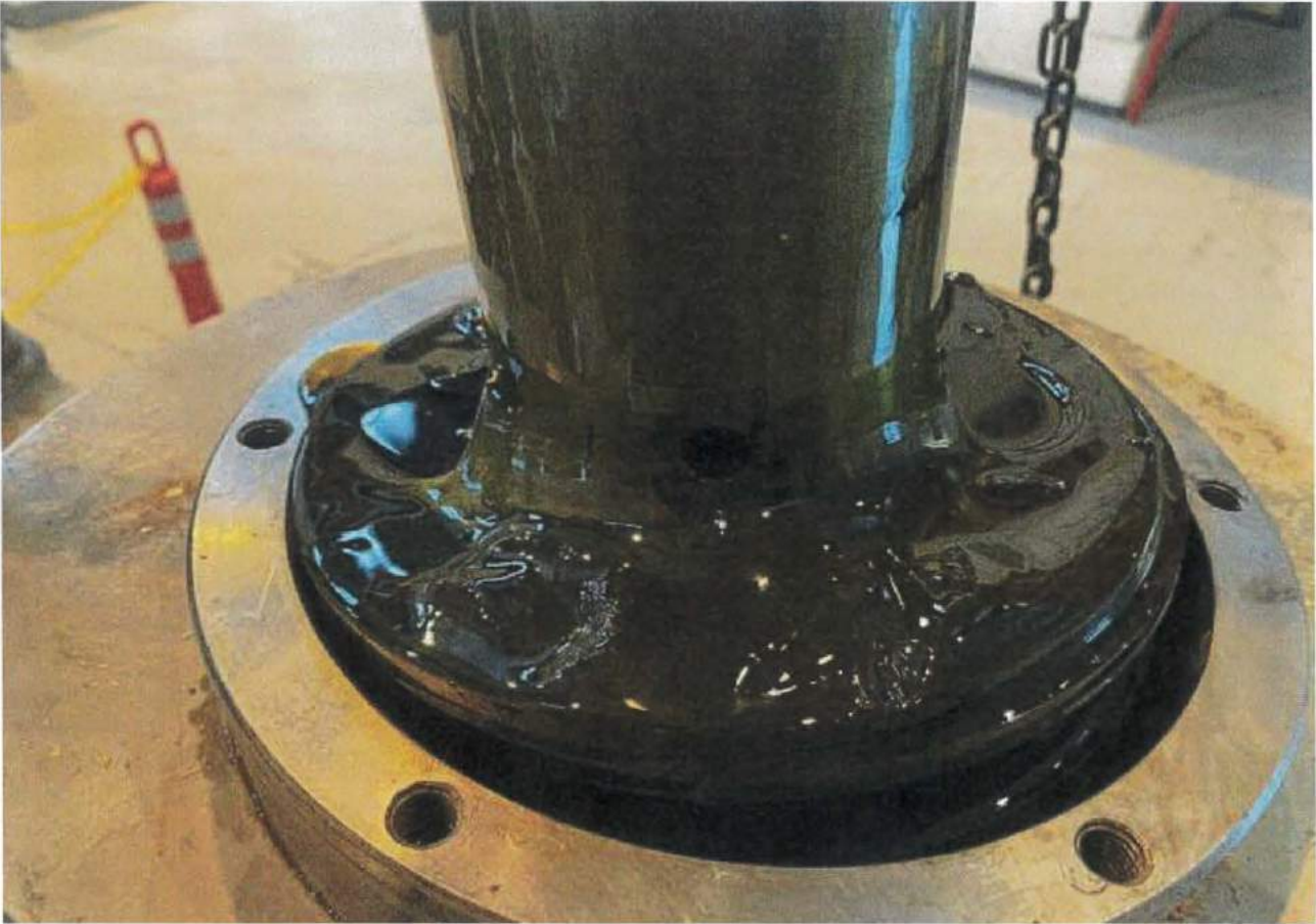
As found inside bore of dashpot cylinder assembly (20).
