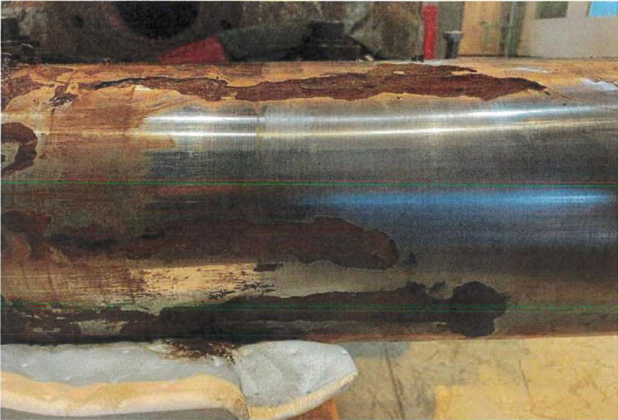
As found lower portion of dashpot cylinder assembly.
