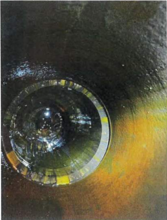
As found inside bore of dashpot cylinder assembly (20).
