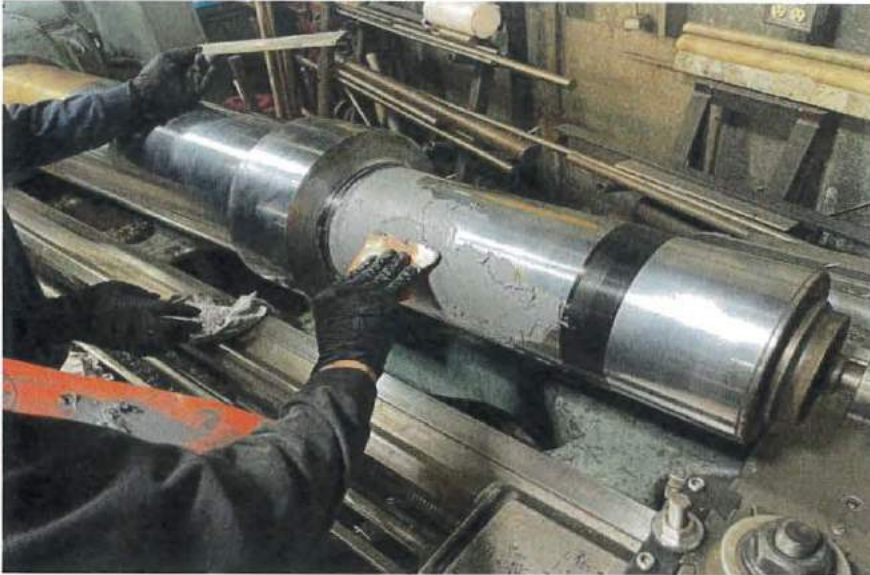
Application of Belzona 1111 onto Dashpot Cylinder assembly.
